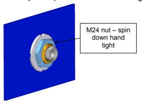
4. Locate the flat spanner into the 4 features on the outside diameter of the washer. Align the jets in the inlet valve by ensuring the arrows on the spanner are orientated along the axis of the tube.
