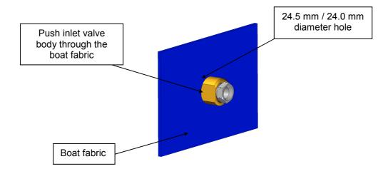
2. Place the washer over the M24 x 1.5 thread, ensuring that the flats line up.
