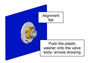
3. Locate the nut onto the inlet valve body and spin down the thread. Tighten hand tight.
